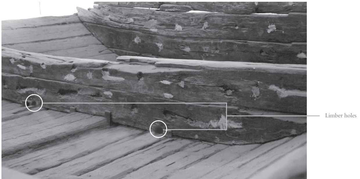
Figure 2.4 The limber holes of the Penglai ship. (Produced by authors)
