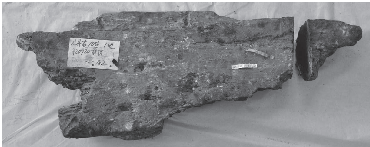
Figure 4.5 A cut piece from the SW-82-182 for metallographic analysis. (Photo by Jun Kimura)
