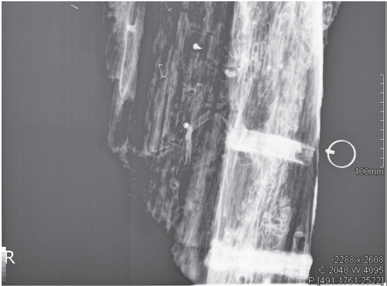
Figure 4.3 X-ray image of the SW-82-182 showing the two iron nails that have square cross-sections. (Courtesy of the National Research Centre of Marine Cultural Heritage)
